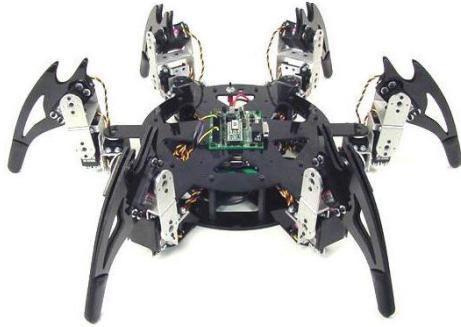
Most often, hexapods are controlled by gaits, which allow the robot to move forward, turn, and perhaps side-step. Some of the most common gaits are as follows:
