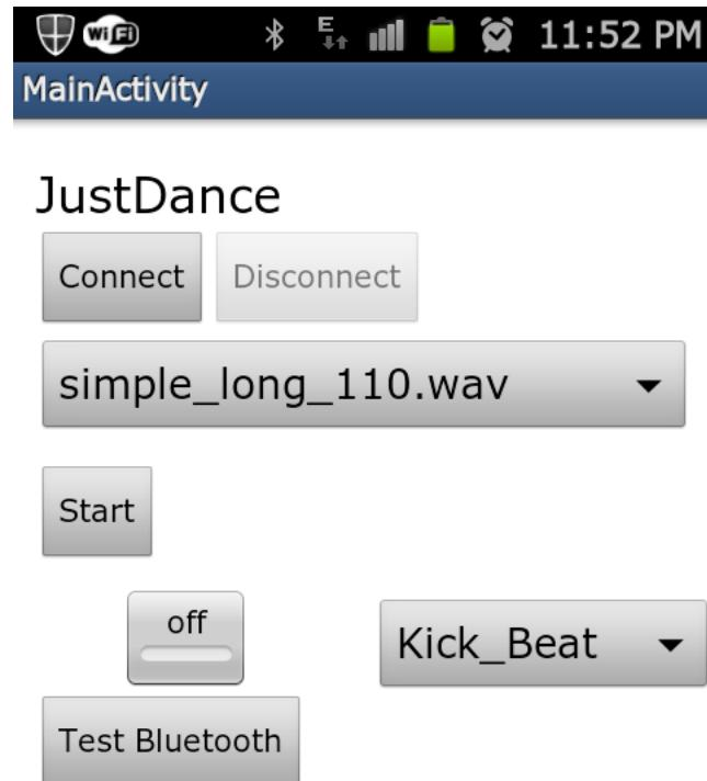
The user interface consists of a Connect and Disconnect button through which the user can connect to or disconnect from the hexapod. The MAC address of the Bluetooth module on hexapod is used to identify the device.
